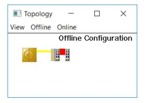
The embedded PC CX5020 (-A1) is displayed within TwinCAT 3 only through the internally installed interface card EK1200-5000.
