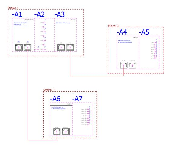
If multiple EtherCAT networks exist in a project, it is required that all networks are additionally defined as logical networks.
